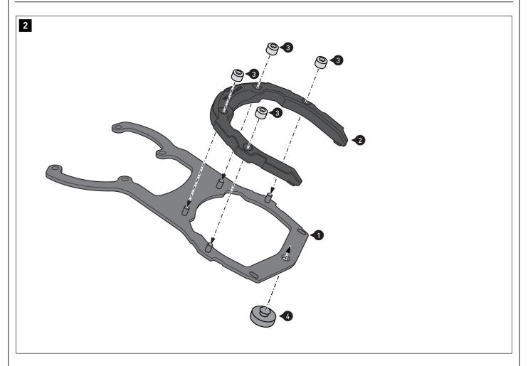
Insert the vibration dampeners (4) into the indicated opening in the mounting bracket (1).
