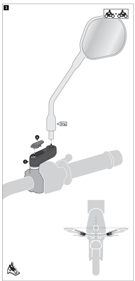
Screw the original mirrors (Orig.) to the mirror extensions (1) using the original parts. Ensure that both mirrors (Orig.) are aligned so that both sides are level.
