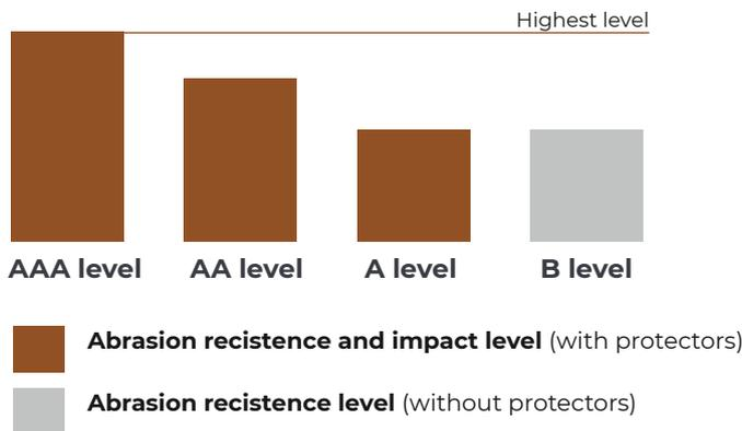
**Abrasion tests** are performed on the construction at three different **zones** (all layers together) of the garment, excluding the detachable linings. The demands vary in these different parts of the body. Shoulders, elbows, hips, and knees have higher demands than for instant inner thighs or underarms.
